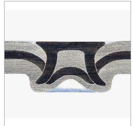
So, Volvo tested a cab assembled with HSPR, without reinforcement plates. The system survived for twice the normal test period without failure. Problem solved.
