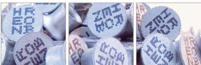
‘self-pierce technology does not generate heat, sparks, fumes, dust or excessive noise’
