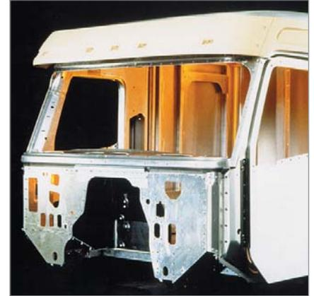
Next was Volvo's FH12 truck cab. The cab used relatively thin, high-strength steel to reduce weight. Spot-welding resulted in fatigue failure during testing.
