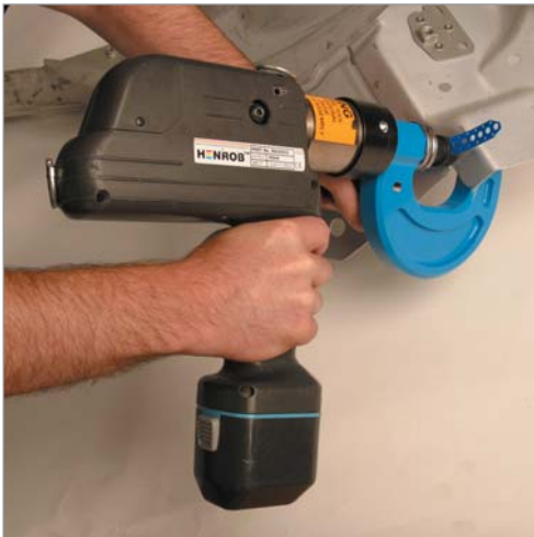
The RivLite handheld tool
