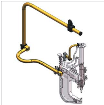
Manually operated tool using a multi axis hanger and twin handed controls.
