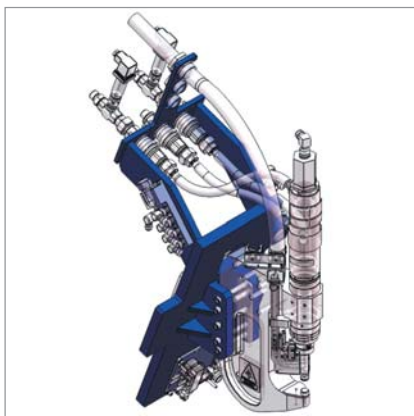
Robot mounted tool incorporating specially designed bracket.
